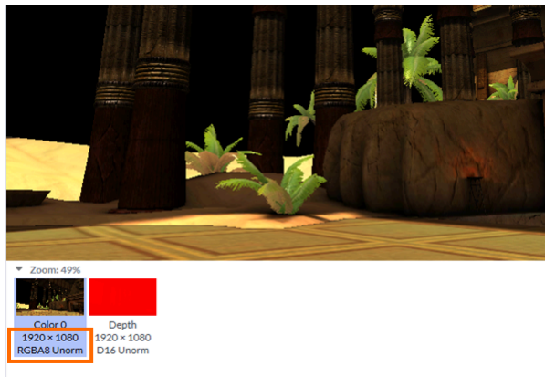
Figure 3-9: Format and data type of framebuffer attachments
